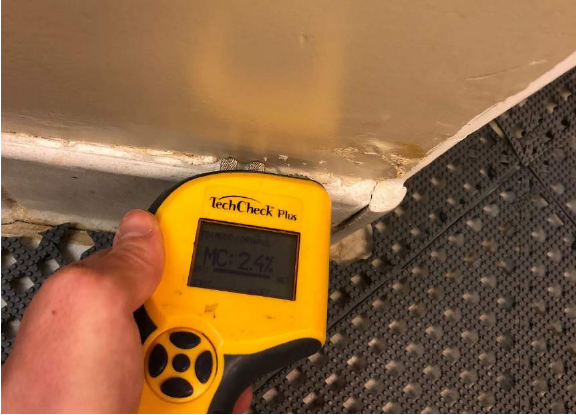
Photograph 4 – Moisture content of 2.4% at Location A which indicated the drywall was wet.
