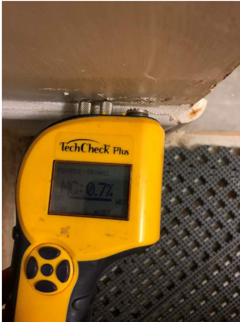
Photograph 5 – Moisture content of .7% at Location B, which indicated the drywall was wet.
